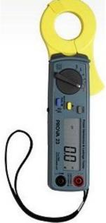
**AC Current** (Auto Range, True RMS, Crest Factor<4, CT=1, Max. peak values 880mADC for mA range, 73.5ADC for A range, Overload Protection AC 600A)
